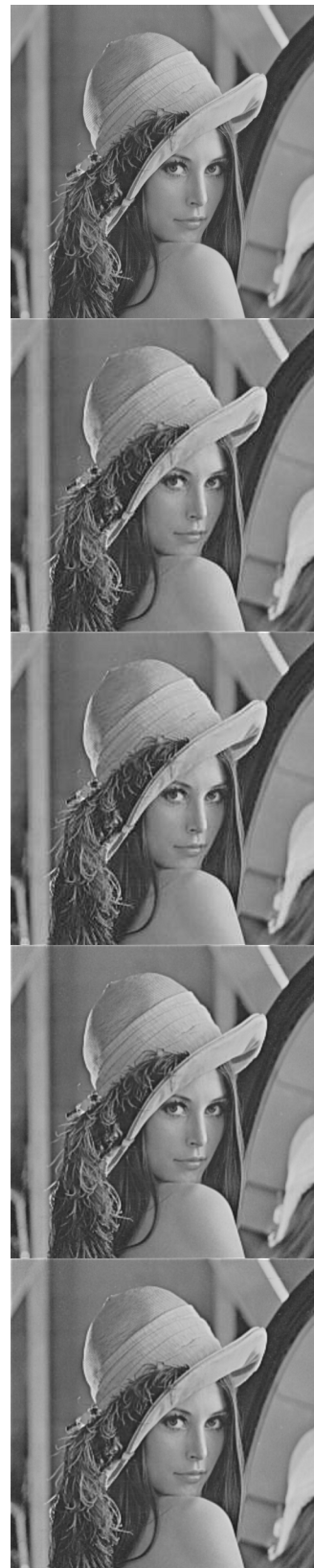
Fig.18: First (top) original image, second (coded and decoded with JPEG), third (coded and decoded with JPEG+Supercompression), fourth (coded and decoded with JPEG2000), fifth (down, coded and decoded with JPEG2000+Supercompression).
